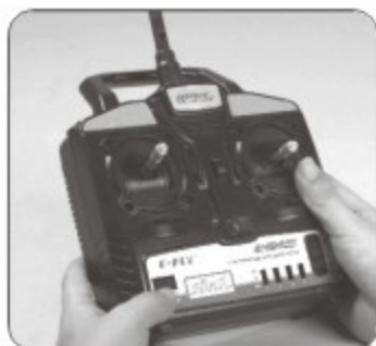
4. Press frequency bind button again to get it rebound. The transmitter get into working mode.
