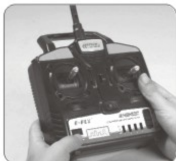
1. Press the button for frequency bind, then turn on the transmitter's power.
