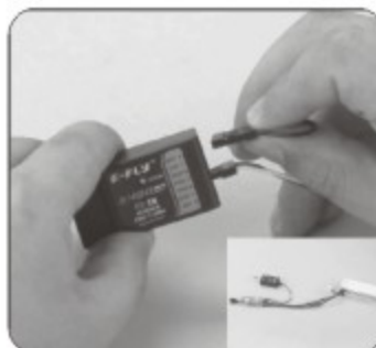
2. Connect the ESC to receiver for electricity supply, which results to the indicator light glitter. And then plug the short-circuit plug into the Receiver in the position of BATT.
